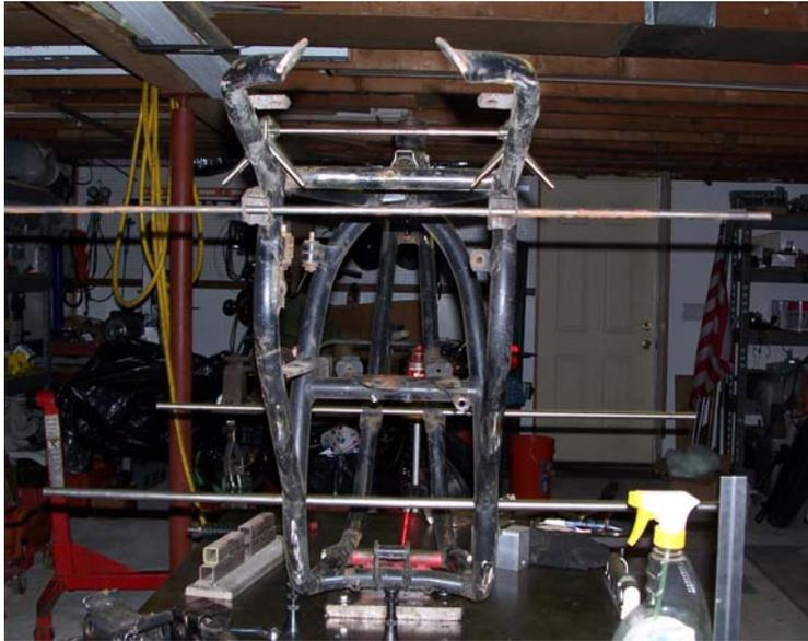
Now between the laser and the drill rod I can see that the swing arm mounts are off the shock mounts are bent badly and the whole frame is actually twisted a little.
