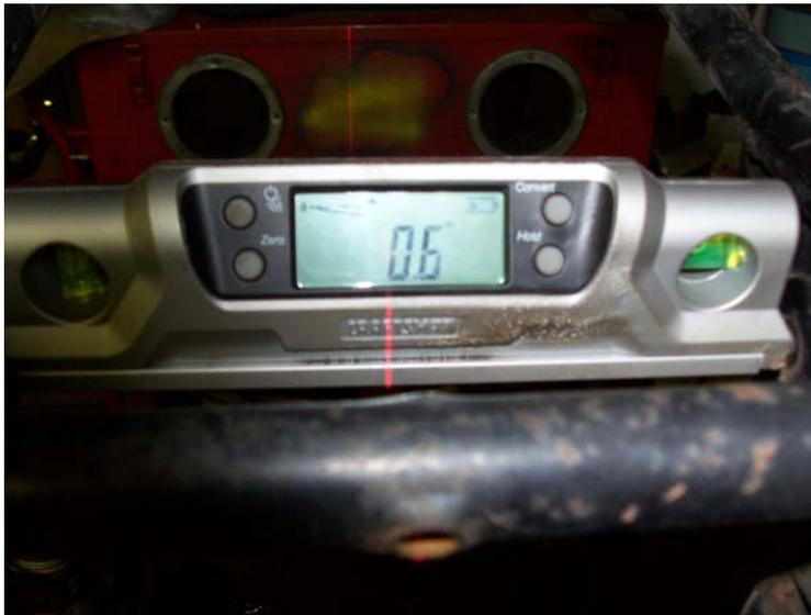
the normal wear of the jig allowed the frames to be off a little here and there. Because of the twist the neck is tilted to the right and the swing arm to the left. I'm not real worried about the shock mounts that a pretty easy fix. The swing arm offers a interesting opportunity though, the bikes handling would benefit from the mount being moved up about a half an inch. Well that's as far as I can go this weekend house needs some work to, I'll add more as the project continues.
