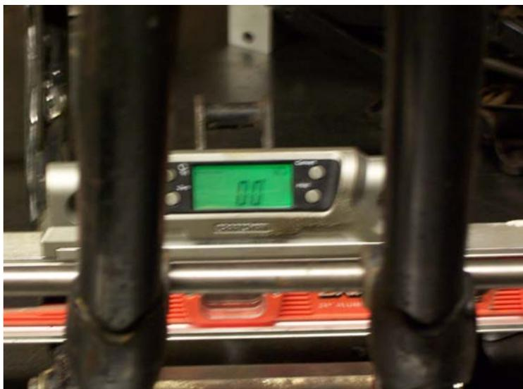
The table has a grid engraved into it which allows me to set up a self leveling laser that shots down the table and from floor to ceiling. I have a jig that bolts to the table and than to the lower motor mount, the jig is centered on the grid so now the frame is centered on the table. I then spend a good amount of time making sure that the frame bolts into the jig level before I start measuring.
